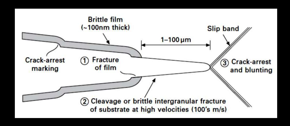
crack growth is discontinuous and that crack-arrest markings should be present on fracture surfaces
